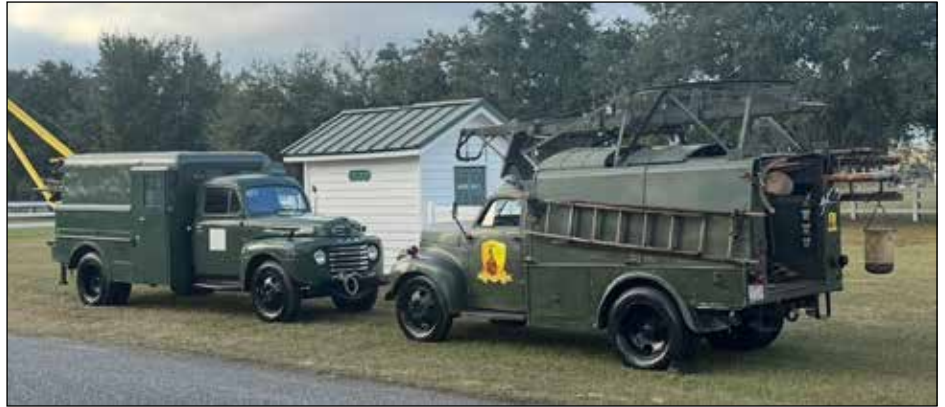
1940's era "A-Frame Pole Setter and a 25-ft. Ladder Truck.
